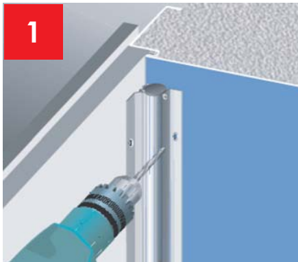
Drill pilot holes for A roller system housing
